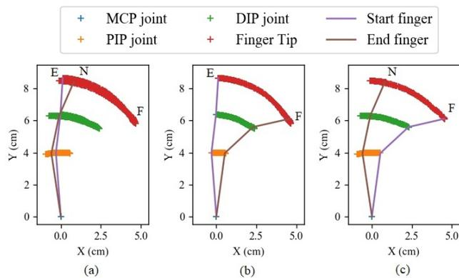
Fig. 4: Upper limb anthropomorphic device actuated finger trajectory showing (a) complete cycle ranging from flexion to extension, (b) flexion action, and (c) extension action.
