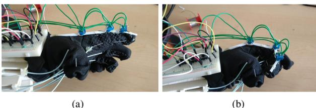
Fig. 2: Pictures of potentiometers interfaced to the upper limb anthropomorphic device to measure finger bending (a) during an extension, and (b) flexion actions.
