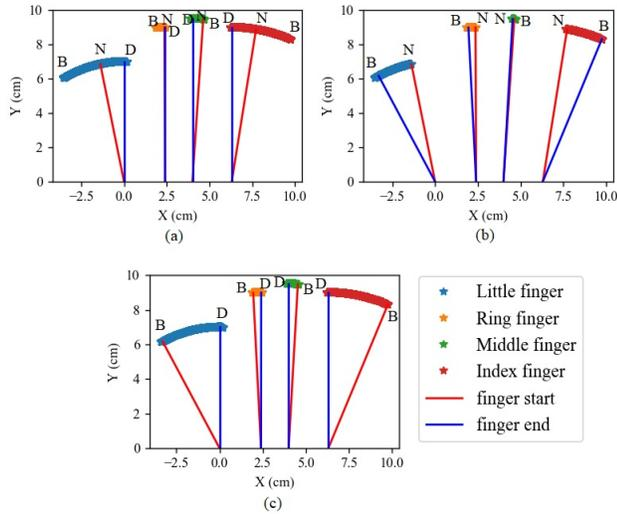
Fig. 5: Upper limb anthropomimetic device driven radial trajectory of four fingers of right hand showing (a) complete cycle ranging from abduction to adduction, (b) abduction motion, and (c) adduction motion.
