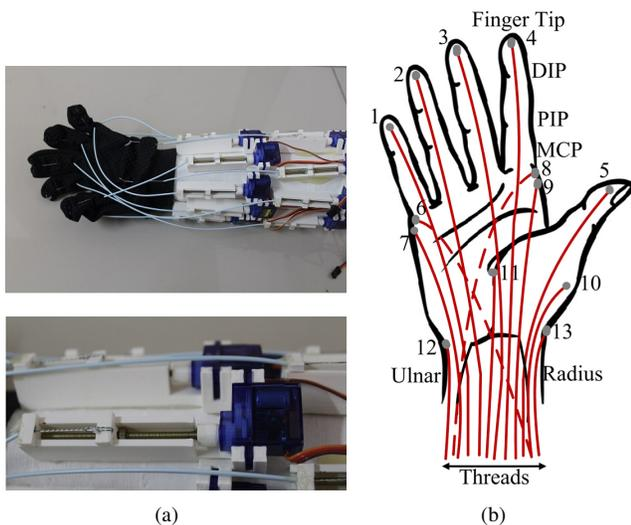
Fig. 1: (a) Pictures of the 3D printed anthropomimetic upper limb assistive device. (b) Schematic representation of anthropomimetic upper limb device showing threads of pulley system, connecting to different parts of glove covering human hand.
