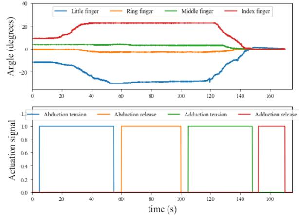
Fig. 6: Anthropomimetic upper limb device generating transient displacement of four fingers during the radial abduction and adduction motion is shown.
