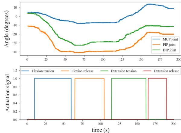
Fig. 3: Transient index finger movement, driven by upper limb anthropomorphic device, showing a complete range from extension to flexion state, as measured by the potentiometers arranged on the joints.
